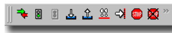
Figure 3.1 Toolbar with the debugger commands (from left): Synchronize, Run, Stop, Step Into, Step Out, Step Over, Go Until, Set Breakpoint, Clear Breakpoint.
