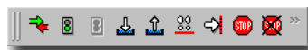
Figure 3.1 Toolbar with the debugger commands (from left): Synchronize, Run, Stop, Step Into, Step Out, Step Over, Go Until, Set Breakpoint, Clear Breakpoint.
